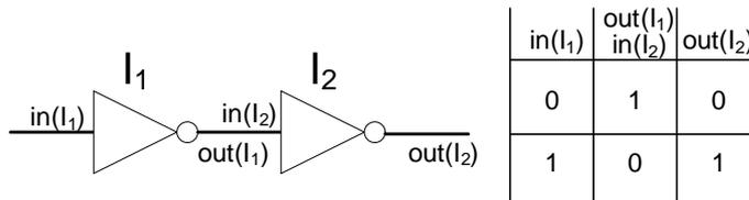
Figure 3. The two-inverters circuit and its normal behavior
