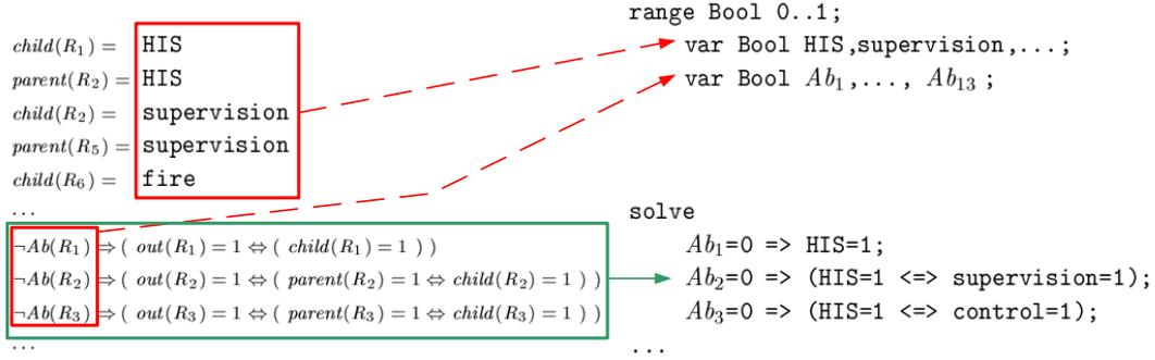
Figure 10. Transforming diagnosis model in Figure 9 into a CSP
