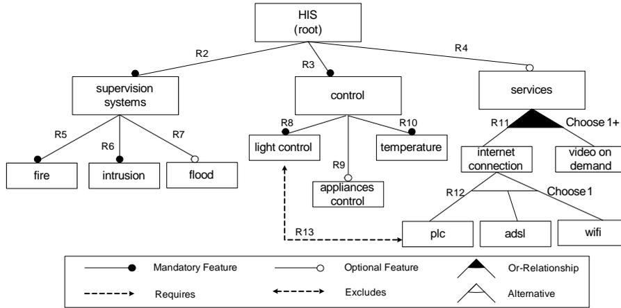
Figure 2. Home Integration System (HIS) feature model diagram
