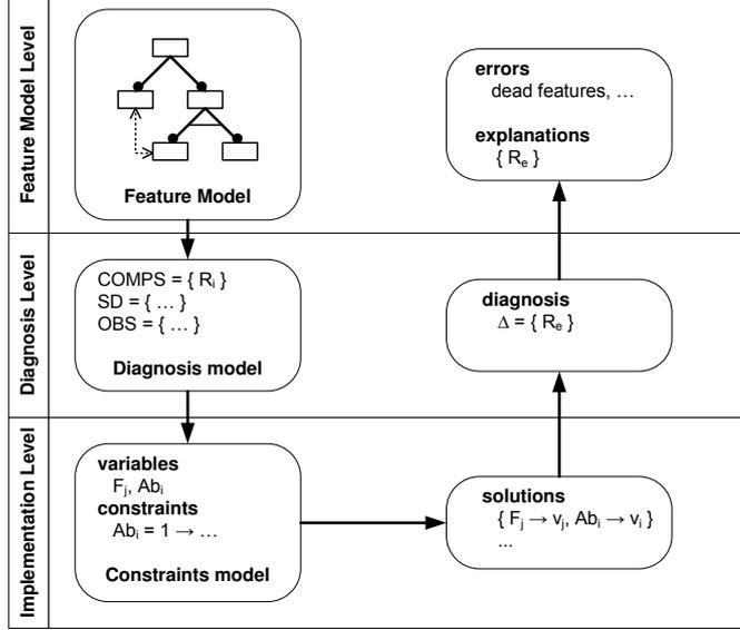
Figure 1. Feature model error treatment framework
