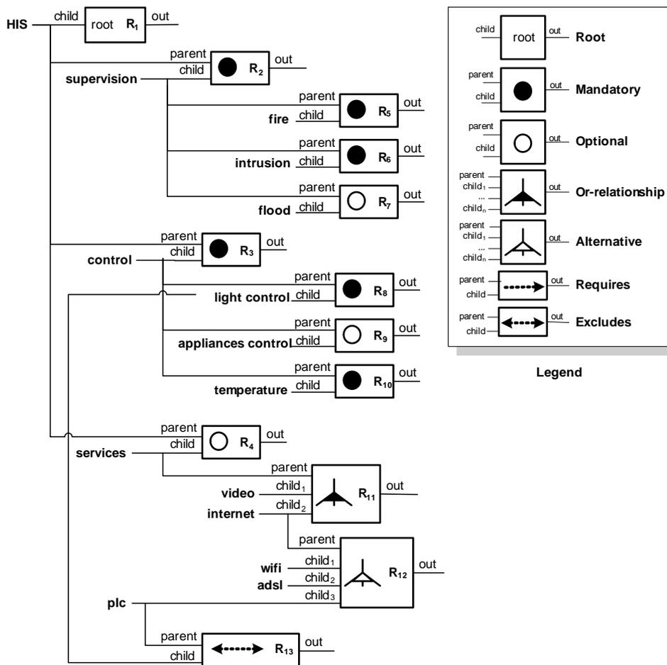
Figure 7. Circuit-like representation of the HIS feature model
